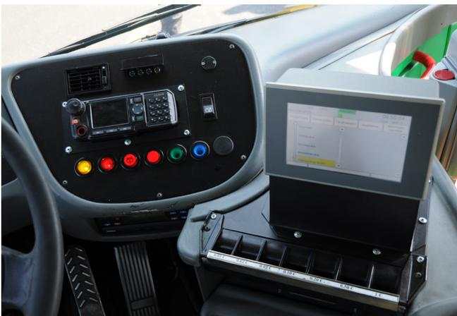
State-of-the-art on-board computers provide drivers with information and manage the entire vehicle periphery in all vehicles.
