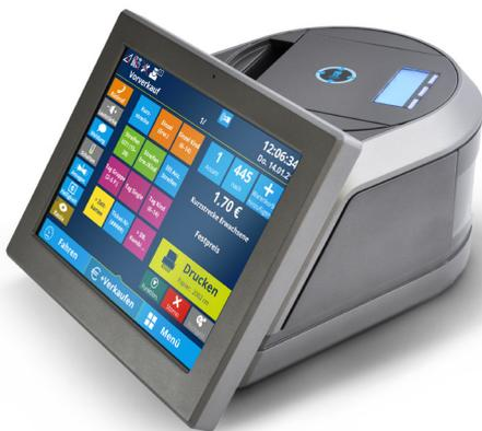
The IVU.ticket.box is the digital control centre in the bus. It records all processes, communicates with the control centre, prints tickets, and validates e-tickets.
